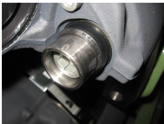
Fig. 2: NEW Knorr Sn6, Open sleeve slide pin
